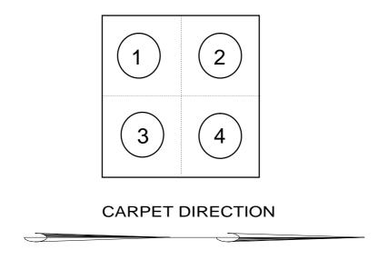
To properly locate the outlets in the floor structure you must review the shop drawing, locate each outlet, identify which outlet position / positions are required for that location and place the appropriate panel in that location. The shop drawing does not indicate the "Powerport " position number.
