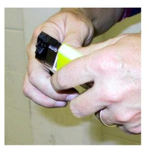
Picture 9-15 Completed Color Coding of Cable Assembly
