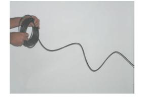
Wrong !!! Pulled off the coil and pulled straight, will result in damage to the cable.
