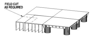
Picture 6-3 Installing the System around obstacles not in starting corner, maintain corner to corner alignment with whole panels and filling in open spaces with appropriate components.
