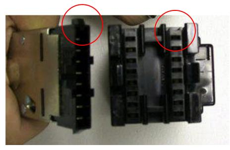
Picture 9-12 Installed Cable Assembly to Junction Block Clip shall be firmly hooked on catch tab
