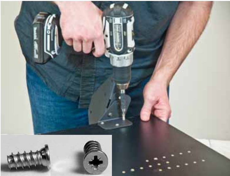
Each iLid mounts with a spring-loaded hinge and a passive hinge.
