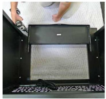
Eight #2 Phillips drive wood screws are provided with the flipIT Kit for installing the keyboard tray.
