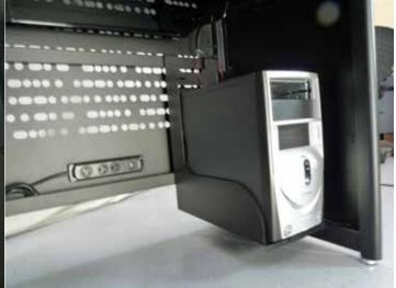
It is best to have the CPU available for making the final installation. If the IT integrator will be doing this part of the installation, have the lock nuts loose enough for them to make this final adjustment.
