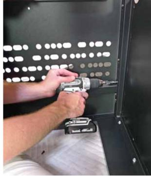
Use four machine screws to install the CPU hanger bar to the base end panels with #2 Phillips drive screw gun.
