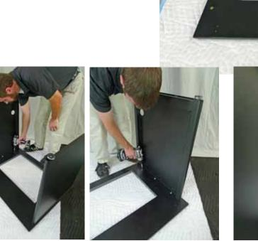
Poition base panels over inserts with wire management holes on the modesty panel side. Use 1/4-20 hex head /#2 Phillips drive bolts to loosely install the base panels; three for each panel. (See below, as to why the bolts are installed only about half way).
