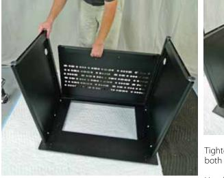
Flex the loosely installed base panels to permit capture of the machine screws by the modesty panel.
