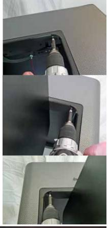
Six #2 Phillips drive wood screws are provided with the flipIT Kit for installing the collar. Three are installed in the left front side to provide added support for the pneumatic cylinder. The other three corners take one screw per corner.
