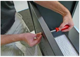
Use two machine screws with lock washers and nuts for installing the power strip to the modesty panel
