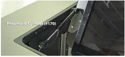
To install the gas spring, or pneumatic cylinder, remove the locking hub, press the end onto the mounting stud, then press the locking hub back into position. The silver shaft end should be lower so it receives lubrication in operation. If it is oriented the other way, the performance life of the gas spring will be reduced.
