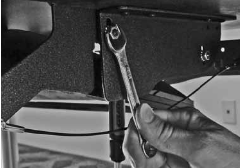
Then remove the monitor to get access to the side adjustments. If necessary, adjust the left and right pivots using the 5/32" hex key and 7/16" open end wrench.
