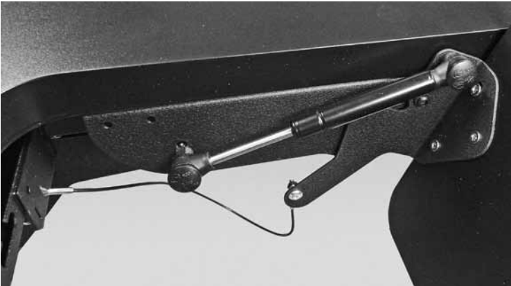
Install the gas spring, silver shaft to the long bracket. Remove locking hub, press end onto post, press in locking hub. Install monitor.
