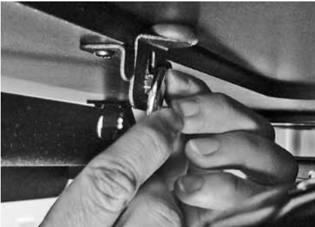
Use 3/8" open end wrench and 5/32" hex key on the rest with the monitor installed.
