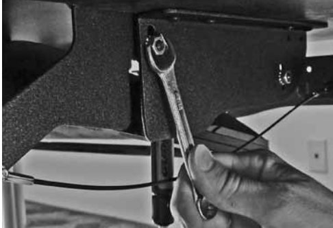
Then remove the monitor to get access to the side adjustments. If necessary, adjust the left and right pivots using the 5/32" hex key and 7/16" open end wrench.
