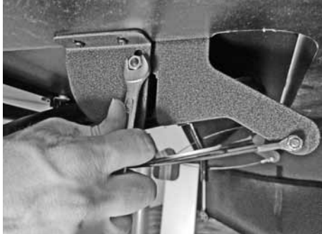
Then remove the monitor to get access to the side adjustments. If necessary, adjust the left and right pivots using the 5/32" hex key and 7/16" open end wrench.
